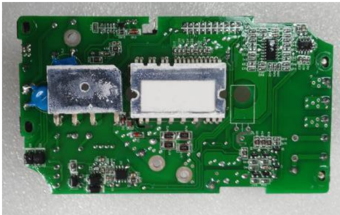
AD100 using the IPM iGBT, but AD350 use Infineon IGBT module
